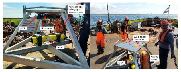
Figure 5.8 RVS frame with Wbat, as deployed in the Marsdiep.
