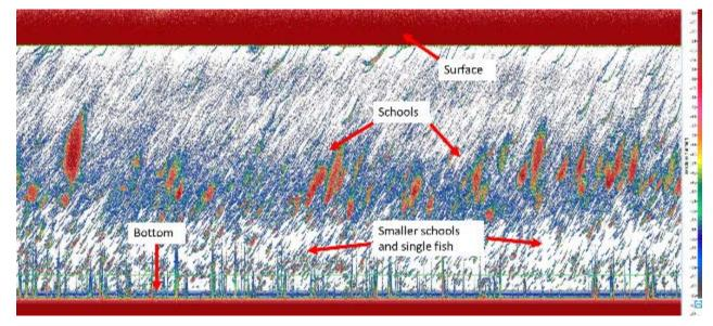
**Figure 5.9** *Example of an echogram from a bottom deployed Wbat, 38kHz. This echogram origins from the Marsdiep area. The depth is 26m.*
