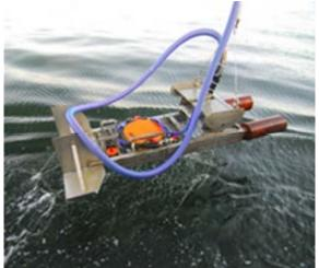
**Figure 5.2** Towed body with 38 and 200kHz transducers. The purple hose protects the electrical cable that is connected to the EK80 in the steering house.
