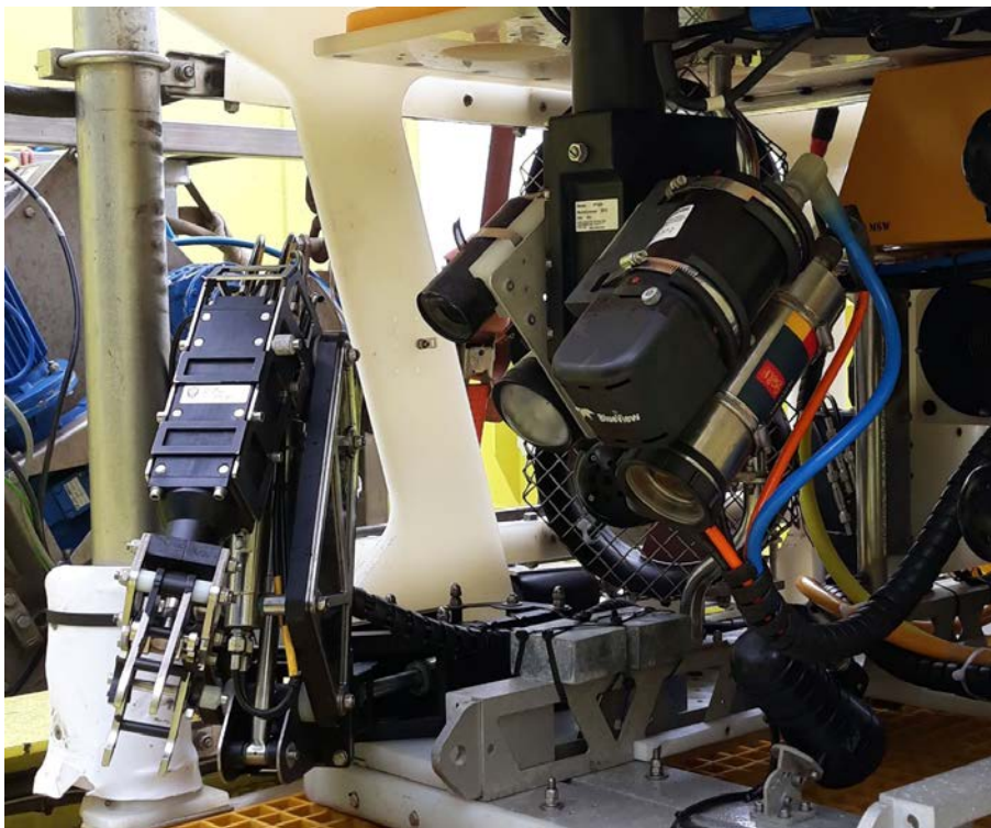
Figure 5.5 Manipulator arm (left) and 4K camera system with video light (right) as present on the Saab Seaeye Panther-XT Plus ROV in use by Rijkswaterstaat. Photo: Joop W.P. Coolen.
