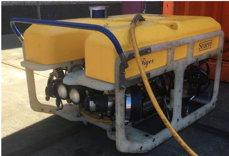
Figure 5.3 Older model Saab Seaeye Tiger ROV, as used in offshore industry for video inspections and small sensor measurements. Photo: Joop W.P. Coolen.
